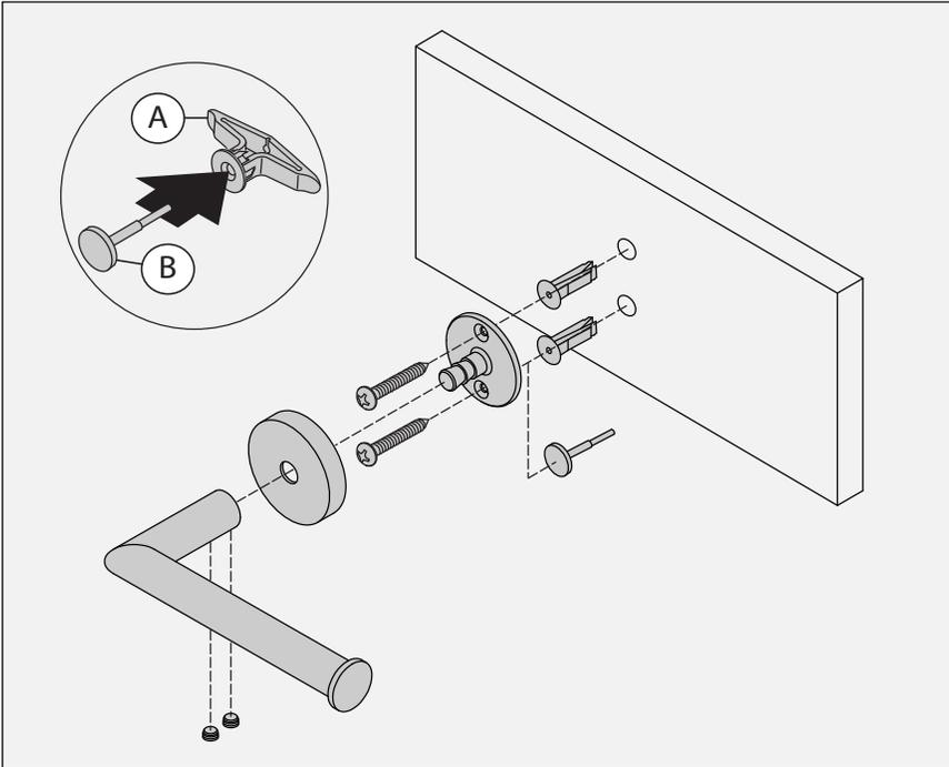
**Note:** For dry wall 1/2" thick or less, insert anchor tool (B) into drywall anchor (A) to secure behind wall prior to installing trim.
