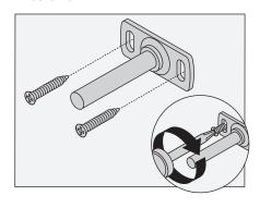
8) Slide accessory into position on bracket and secure with set screw.
