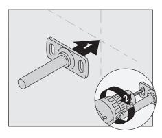
7) With mounting brackets in position, secure to wall using screws.
