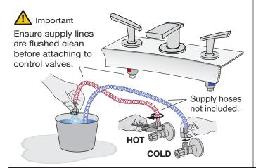
Step 9 Connect supply lines, check for leaks
