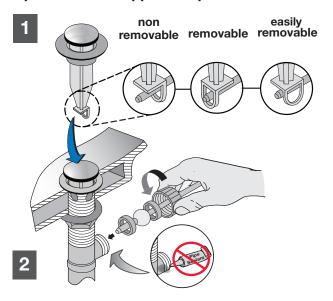
Step 7 Connect lift rod and adjust linkage
