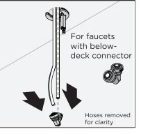
Remove flow restrictor and flush supply lines free of debris. Check for leaks.
