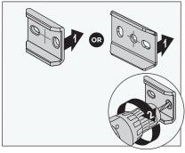
5) Secure with set screw. **Note:** The set screw should be snug, but do not overtighten
