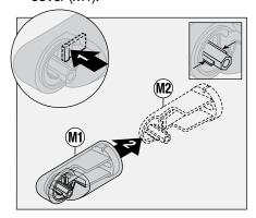
**Note:** Mounting plate (M2) center tabs must be horizontal for removal.
