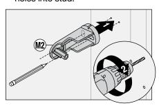
**Option:** Place mounting plate (M2) in position, mark and drill 3/16" holes into wall. Install anchors.
