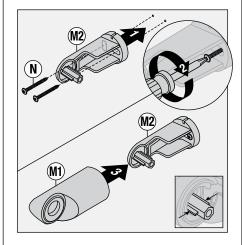
**Note:** Mounting plate (M2) center tabs must be horizontal for installation.
